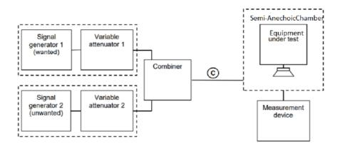
II. General Test requirement – Conducted Measurements
